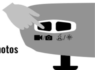
Press the "Photo" button once, the transmitter will sound "di" to take a picture.
