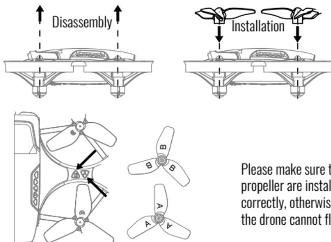
Please make sure the propeller are installed correctly, otherwise the drone cannot fly.
