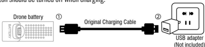
▲ Only use the original charging cable; suggest select Adapters with output current of 5V 2A.
