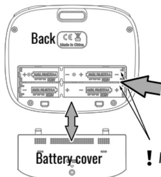
Open the battery cover of the remote controller and place the same type of battery with saturated capacity, according to the '+' electrode indication in the battery cell (Not include).
