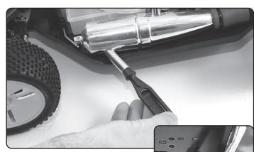
4. Stopping the engine. To stop the engine either use a stop tool to cover the exhaust outlet or use a flywheel stop tool.
