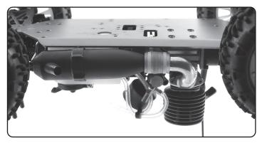
2. Then turn the car upside down and pull the pullstarter rapidly until all the excess fuel has emptied onto the floor through the glowplug hole. Make sure you do this outside safely. This process is really only necessary when the engine is cold or brand new and tight.
