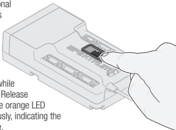
**TIP:** It is still possible to use a bind plug in the bind port if desired. This can come in handy if the receiver needs to be mounted in a location that is difficult to access, in which case a servo extension may be used for binding. If using a bind plug, remove after binding to prevent the system from entering bind mode the next time the power is turned on.
